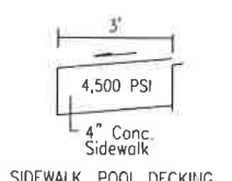
SIDEWALK, POOL DECKING & EQUIPMENT PAD DETAIL N.T.S.
